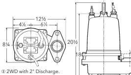
2 WD with 2" Discharge.2 WD with 3" Discharge.
