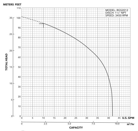
= A 11/4" minimum discharge pipe requires a minimum flow of 10 gpm to maintain a 2 ft./sec. scouring velocity. Flows less than 10 gpm will allow solids to settle in the pipe.
